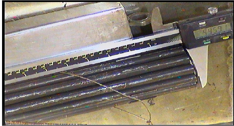
Fig. 1. Shows the fuel bundle length measurement.
