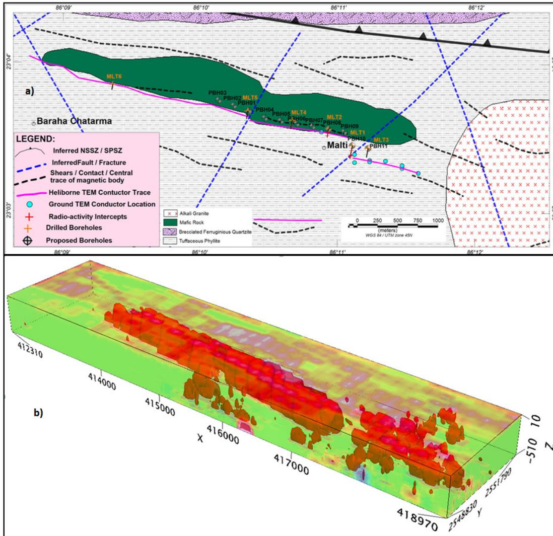
Figure 6 a) Geological map of the Malti area, Purulia district, West Bengal highlighting WNW-ESE conductor b) 3D voxel model with a 150 mS/m iso-surface representing the conducting sulphides/carbonaceous phyllite.
