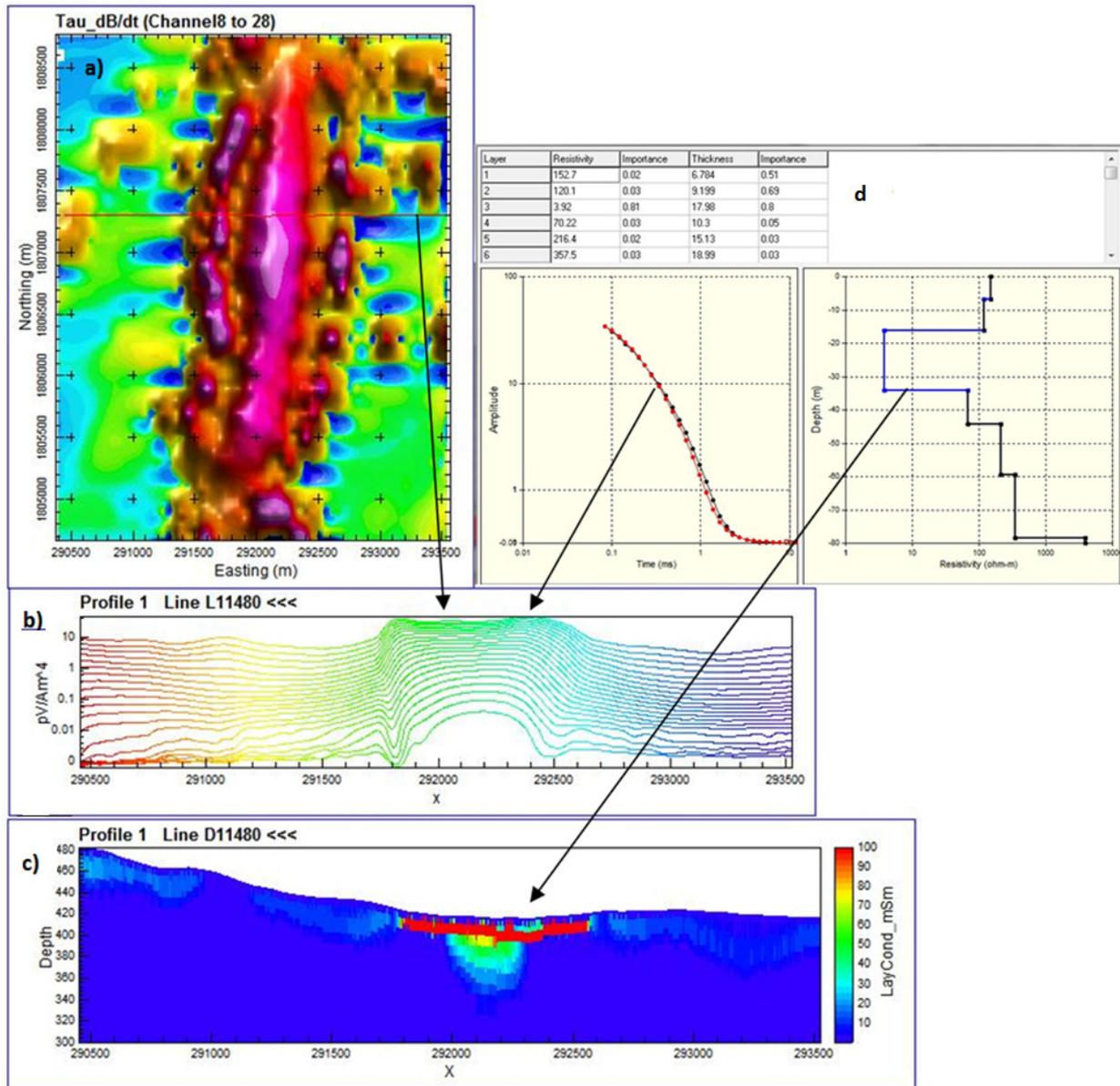
Figure 4 a) Tau image for the target area b)  $dBz/dt$  profiles along the line L11480 c) CDI along the line L11480 and d) Layered modeled response for the transient indicates a low resistivity layer at a depth of 25 m with a thickness of 20 m.
