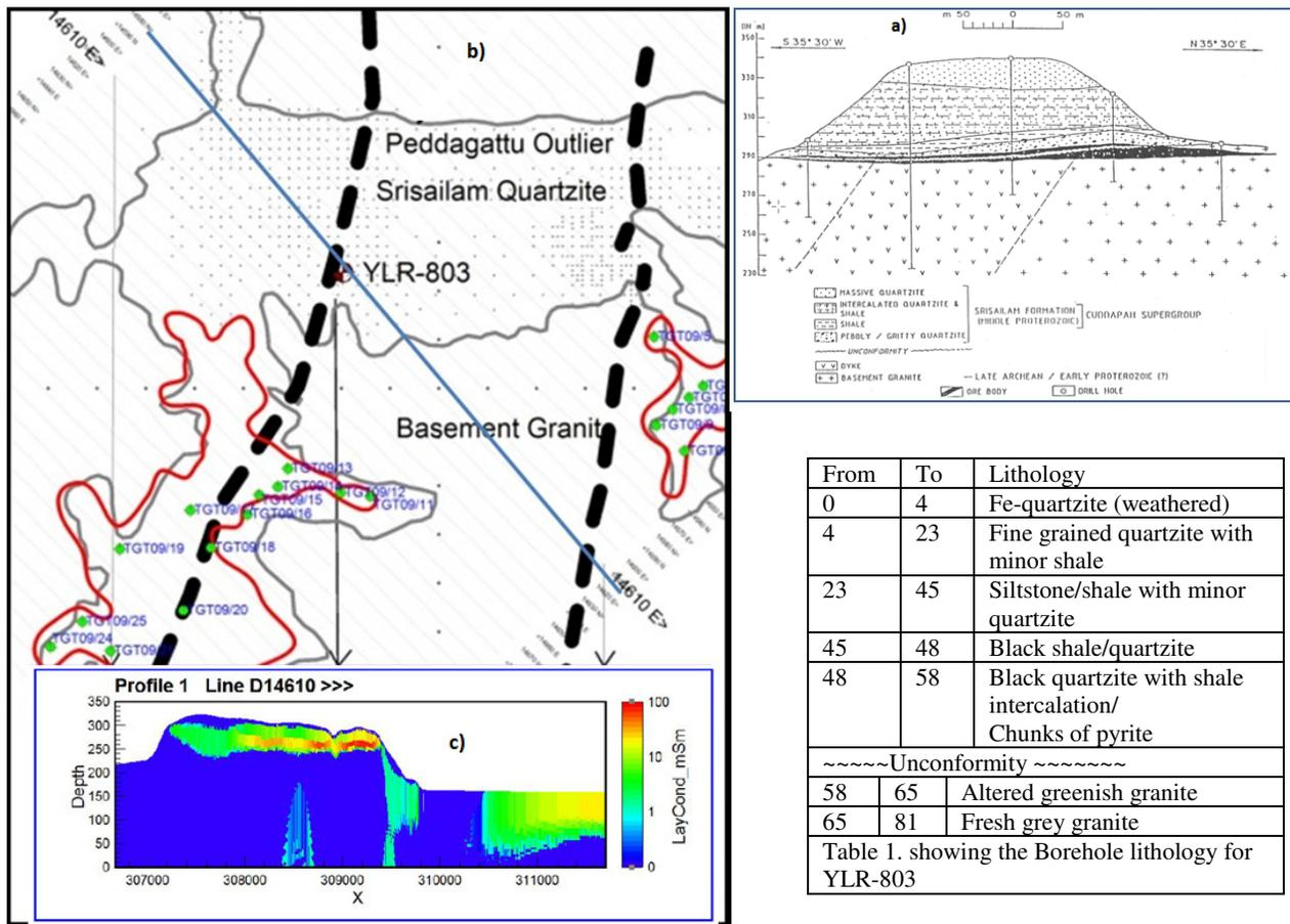
Figure 3. a) Geological cross section across Lambapur outlier b) Geological map of Peddagattu outlier c) CDI along the flight line 14610 (part) highlighting the unconformity.
