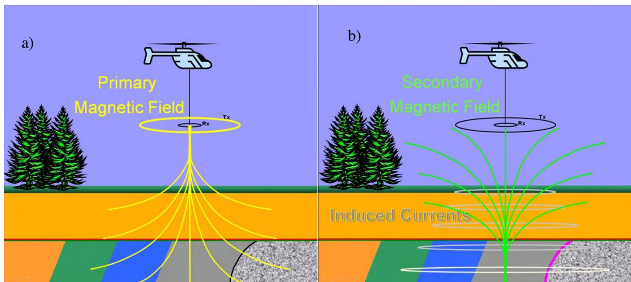
Figure 1. Typical heliborne time domain EM system (Sketch) a) primary magnetic field due to alternating current in the transmitter loop (Tx) b) Secondary magnetic field received in the receiver loop (Rx) due to subsurface conducting geology.
