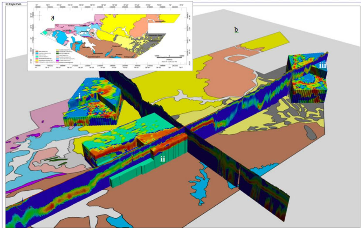
Figure 5. a) Geological map of northern part of the Cuddapah basin (Block-III) b) CDIs along the tie line T90150 and flight line L13500 in a 3D perspective view similar to fence diagram viewing from SE highlighting the conducting layer below the Kurnool group of rocks. Also, 3D voxel chair clip models generated for the three selected areas i) in parts of Srisailam sub-basin, ii) Kurnool sub-basin and iii) Nallamalai sub-basin highlighting the conductivity structure in the area.
