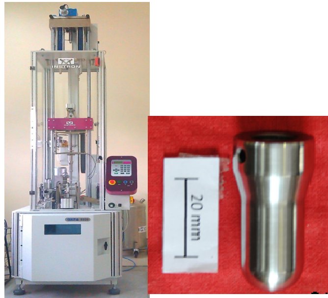
Fig.2: Instrumented drop weight impact tester (Model-9350) and impactor
