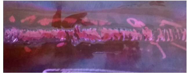
FIG 3: After Penetrant Application.
