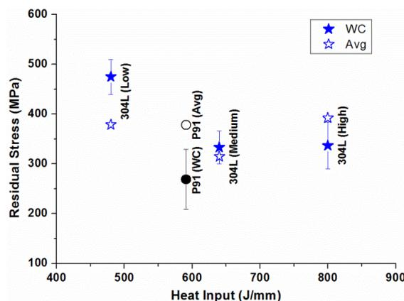
Fig. 3 Variation of residual stress with heat input in SS 304 L and P91 weld pad (filled symbols are indicative of measurements at WC whereas open symbols are for average stress)
