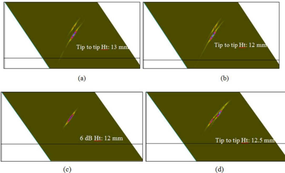
Figure-9: B-Scan image of slot having 12 mm height and oriented at (a) 2.5° (b) 20° (c) 45° and (d) 55°
