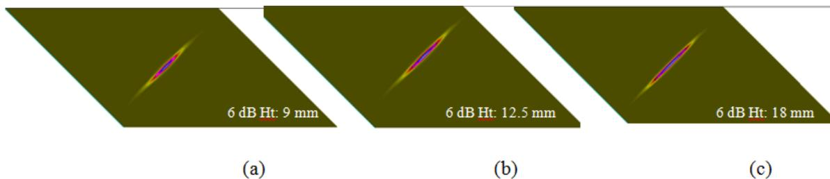
Figure-2: B-Scan results for 45° inclined slot with through wall height of (a) 6 mm (b) 12 mm and (c) 18 mm
