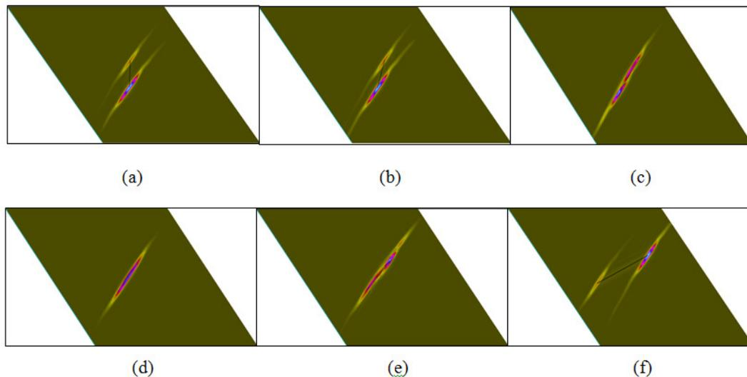
Figure 5: B-scan image of slot having 12 mm height and oriented at (a)  $2.5^\circ$  (b)  $20^\circ$  (c)  $40^\circ$  (d)  $45^\circ$  (e)  $50^\circ$  and (f)  $70^\circ$
