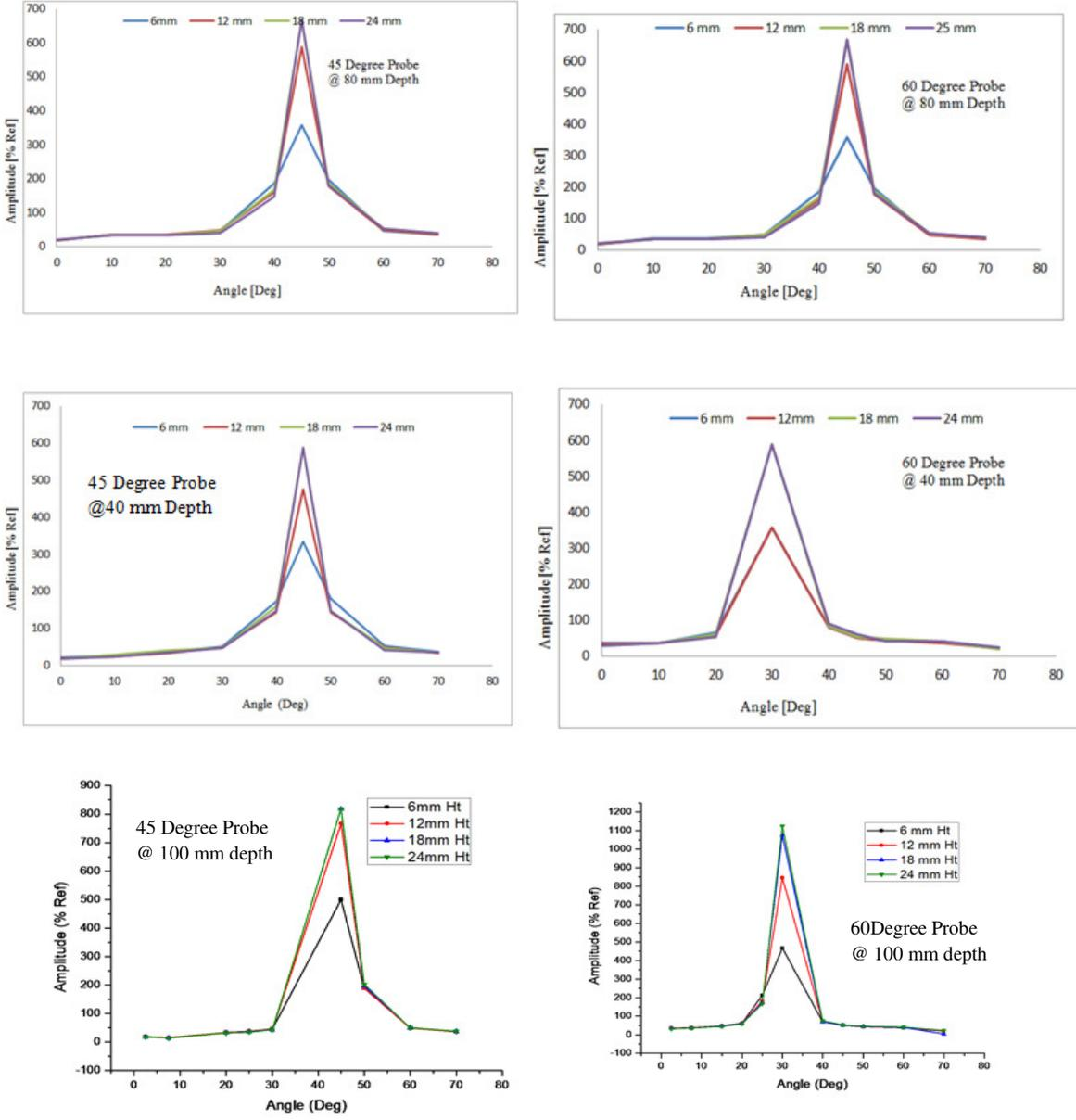
Figure-4: Variation of signal amplitude with flaw orientation for 45° Probe & 60° Probe @ various depths
