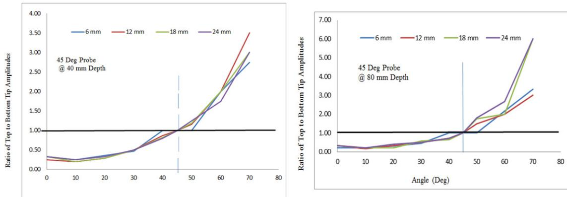
Fig 7: Variation of Ratio of Top Tip to Bottom Tip Amplitudes with respect to orientation
