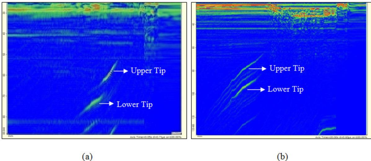
Figure 10: B-Scan Images of 0° slot (a) 45° (b) 60°
