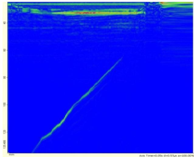
Figure:B-scan image obtained by 60° probe
