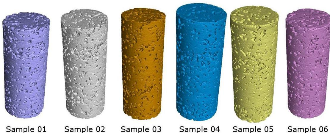
Fig. 5 – 3D CT image of six number of EPC samples scanned using X-ray CT
