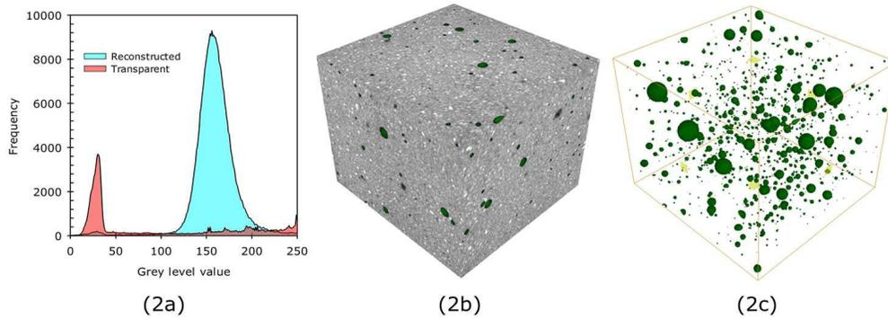
Fig. 2 – a. Adjusted GLV, b. Reconstructed and c. Transparent CT image of the cement paste sample
