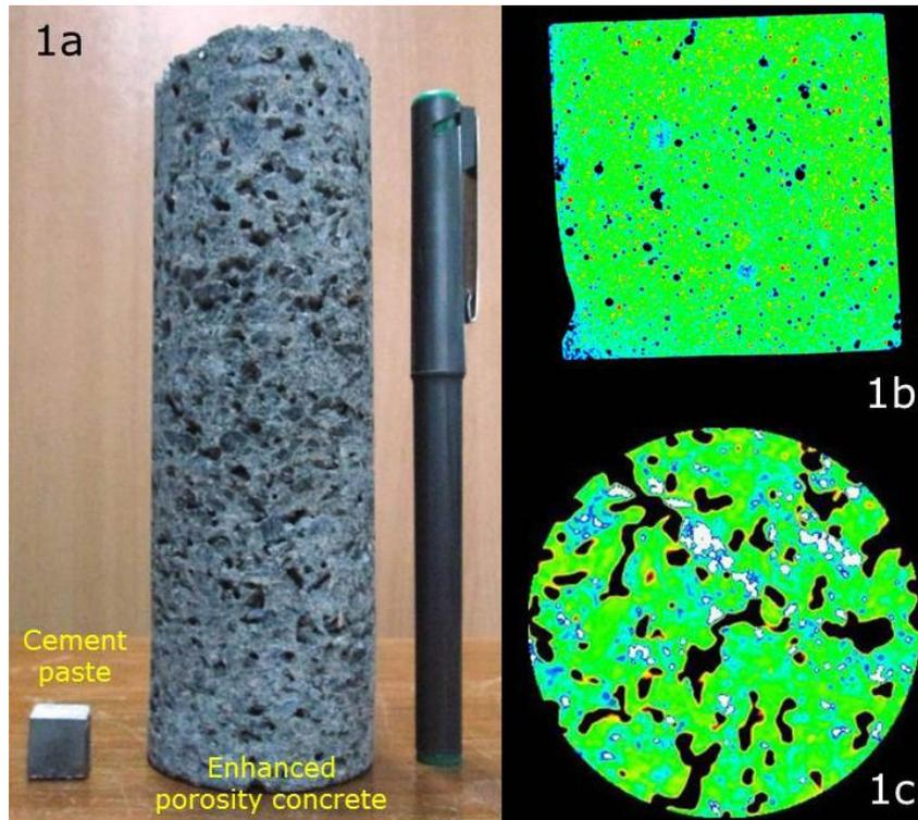
Fig. 1 – a. Cement paste and EPC sample scanned using X-ray CT, b-c. Pseudo-coloured 2D CT slice of cement paste and EPC sample
