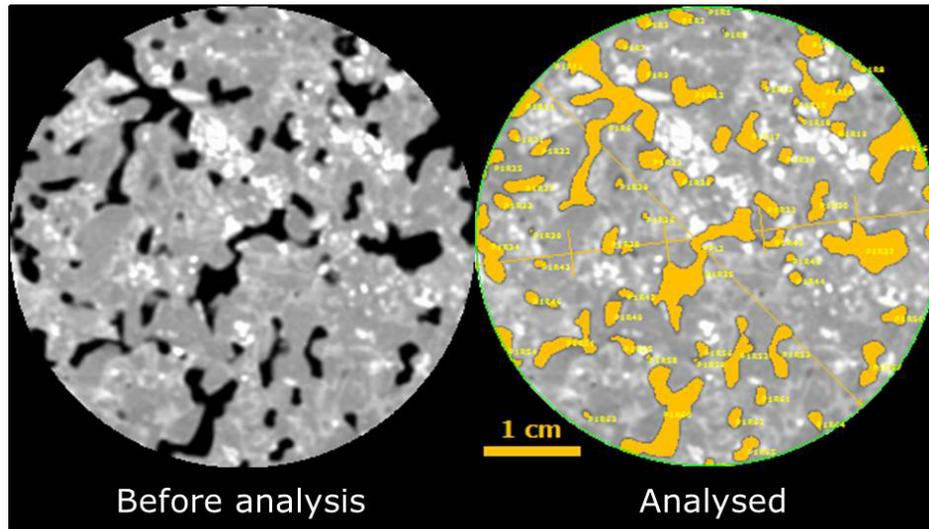
Fig. 6 – CT slice of the EPC sample before and after image analysis
