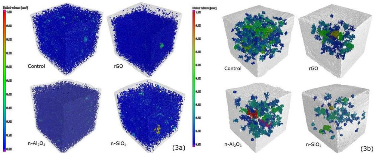
Fig. 3 – Colour-coded transparent 3D images of the different pastes having pore/void volume ranging between a. 0.01 to 0.75 mm<sup>3</sup> b. 0.07 to 0.75 mm<sup>3</sup>
