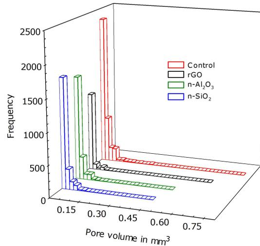
Fig. 4 – Histogram results representing the pore/void volume inside the different pastes analysed using Porosity Module of the software VGStudio MAX 2.2
