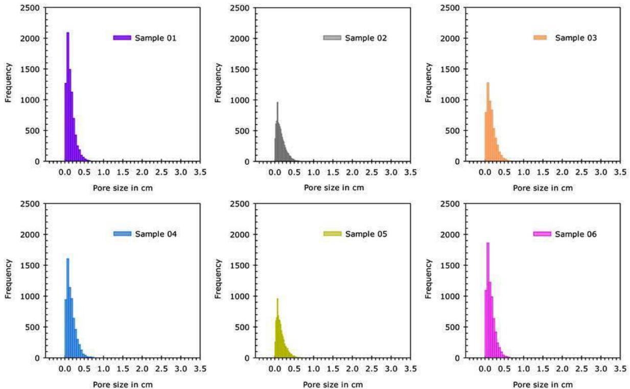
Fig. 7 – Histogram results representing the pore size distribution of the different EPC samples
