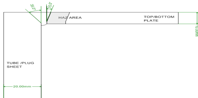
FIGURE-2: WELD GEOMETRY
