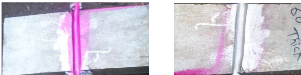
Fig. 3 LP tests on 60 mm TIG welds (no cracks/surface defects found)
