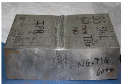
Fig.2(a) TIG weld sample (macro)
