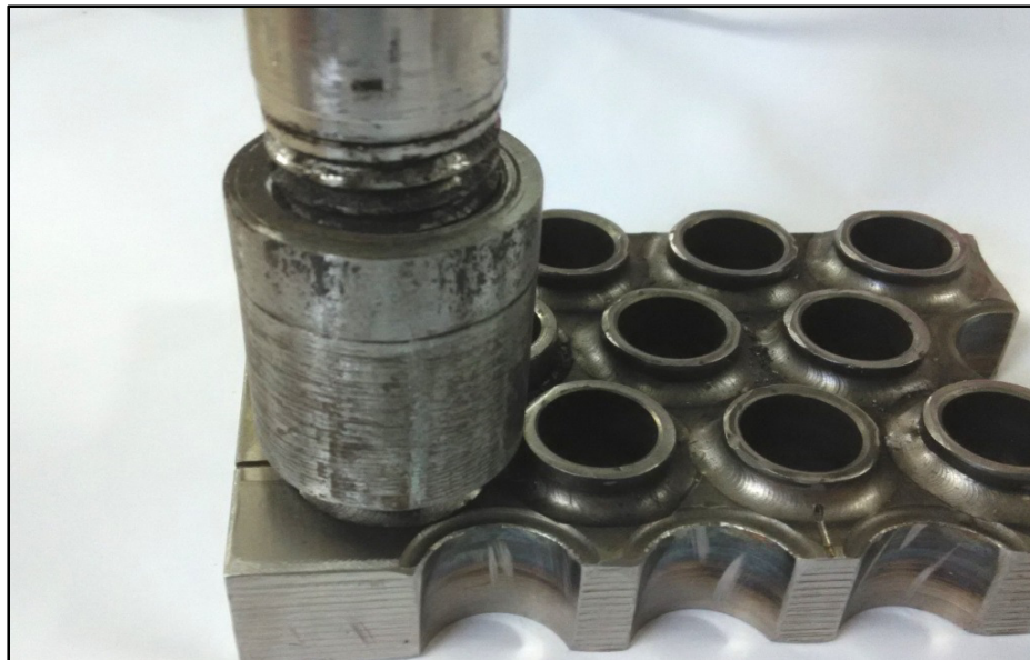
Calibration on 1 mm Flat Bottom Hole
