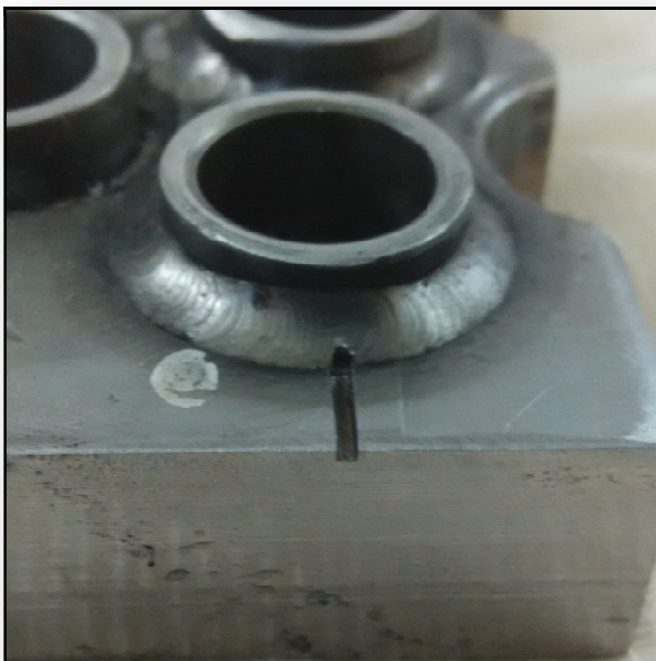
Calibration Block with 1 mm Flat Bottom Hole
