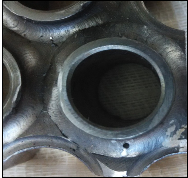
Calibration Block with 1 mm Flat Bottom Hole-Angular
