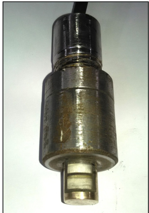
UT probe with Fixture Arrangement
