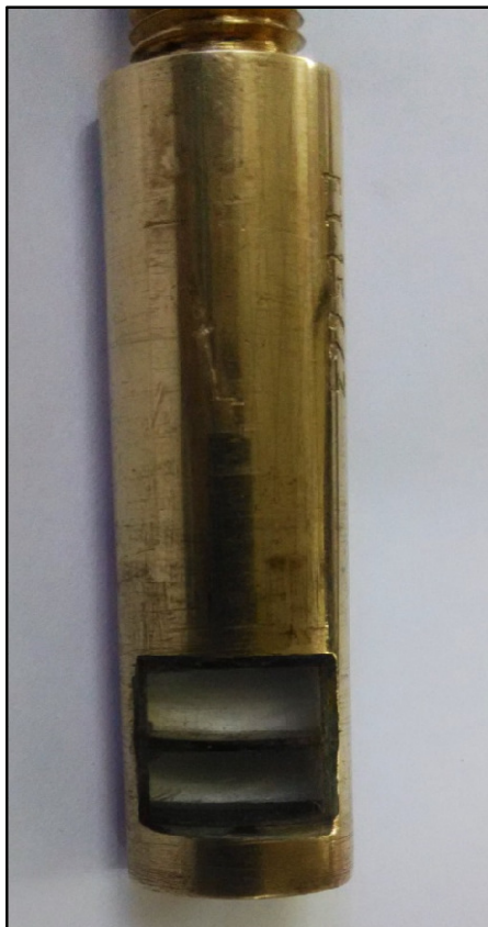
UT probe – Dual crystal, 10 MHz, \varnothing 15 mm
