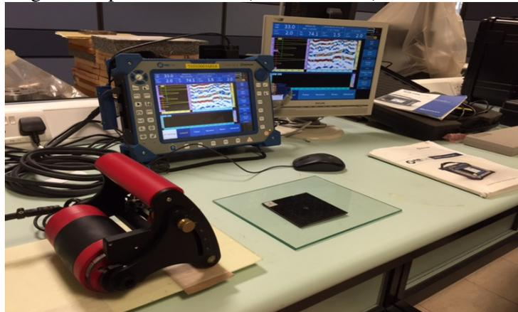
*Fig.1. Experimental setup for Doppler phased array UT testing*
