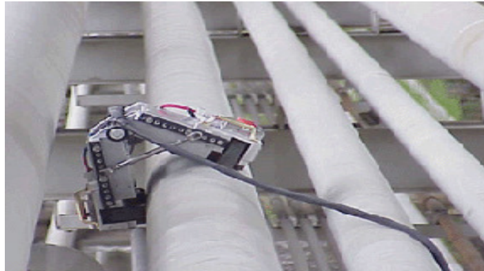
Fig.2. EMAT on a pipeline - Showing the transducer position and a typical set up.
