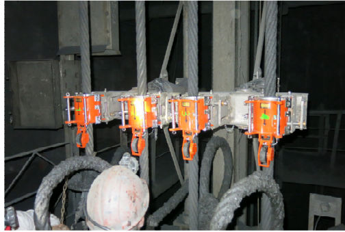
Fig.6. System INTROS to simultaneously inspect 4 mining ropes.
