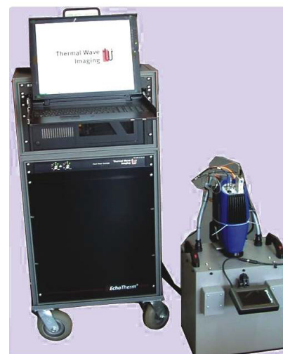
Fig.2. Photograph of pulsed thermography system
