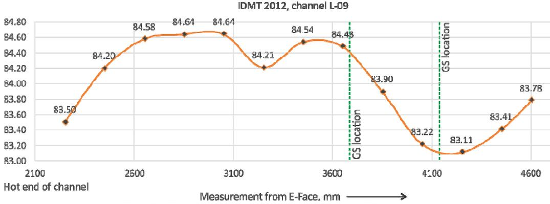
**Fig 3: Typical plot showing dip in ID profile**
