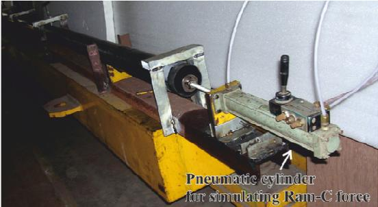
Figure 8: Pneumatic cylinder, for Ram-C force simulation
