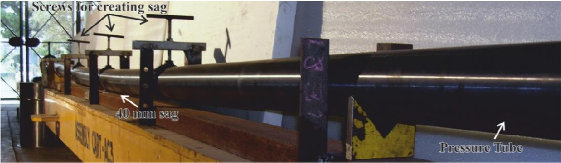
Fig. 7: Sagged pressure tube test setup
