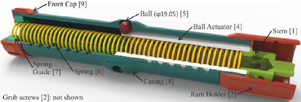
**Fig. 2: IDMT 3D visualization, component number in square bracket**
