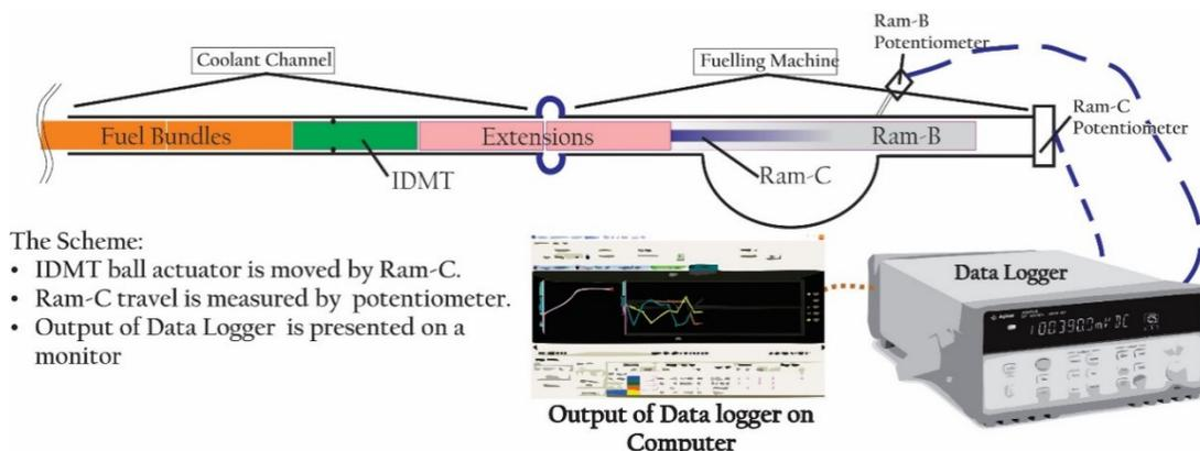
**Fig. 1: IDMT schematic**
