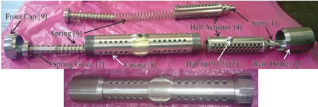
**Figure 5: Recently manufactured compact IDMT components**
