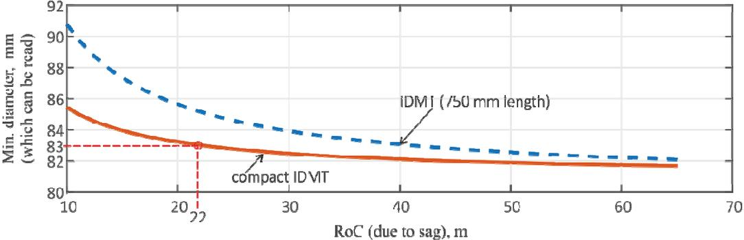
Figure 6: Relation between Radius of Curvature (RoC) and min. diameter required for reading
