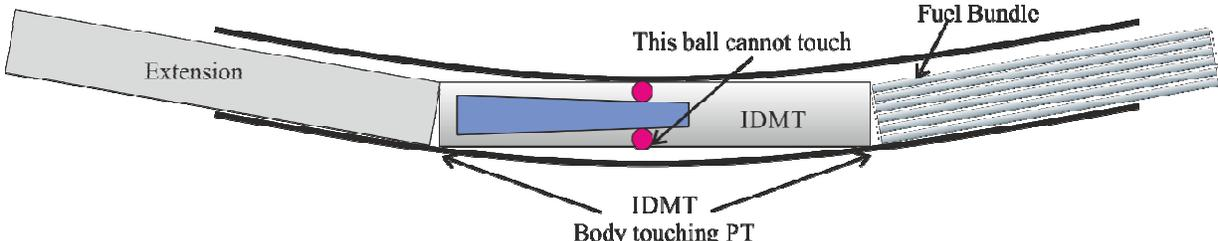
**Fig. 4: Explanation of reading lesser diameter than actual**
