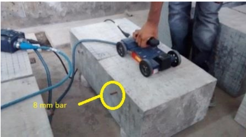
Fig. 5 Data collection on a typical concrete block specimen with 8mm diameter rebar
