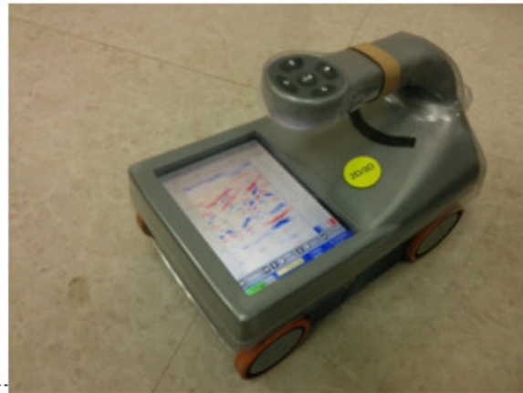
.....Fig. 1(a) GPR with antenna .....| Fig. 1(b) Compact GPR (Structure Scan Mini-HR)¶
