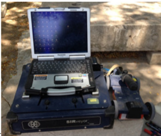
.....Fig. 1(a) GPR with antenna .....| Fig. 1(b) Compact GPR (Structure Scan Mini-HR)¶
